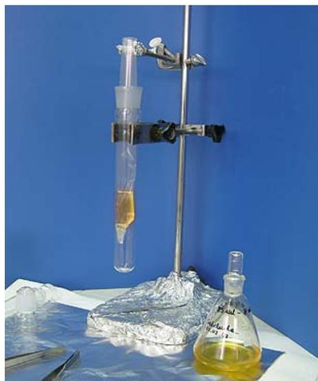
Fig. 2. Diaphragm filled with sample of fat extract
